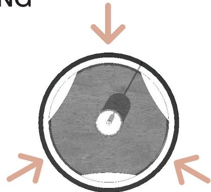
TO LEVEL THE PENDANT - SUPPORT THE TIMBER PLATE FROM THE UNDERSIDE WITH ONE HAND AND WITH THE OTHER HAND, SLIDE THE CERAMIC LAMP HOLDER CUP WITHIN THE CENTRE HOLE OF THE TIMBER PLATE AS REQUIRED.
