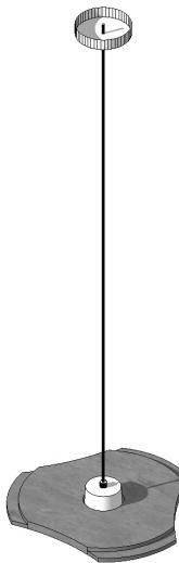
**ATTENTION: NO PART OF THE PENDANT ASSEMBLY MUST EVER BE ALLOWED TO HANG FROM THE ELECTRICAL FLEX. ALL ELECTRICAL CONNECTIONS MUST BE CARRIED OUT BY A LICENSED ELECTRICAL CONTRACTOR.**
